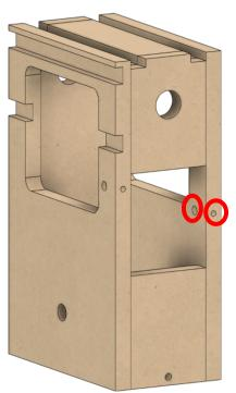
If you purchased the kit we supply, the holes on the left and right are already set properly. If you built it yourself, you will now need to drill the holes for the screws on the right. As noted in the case building instructions, these need to be set based on the alignment of the bracket.
